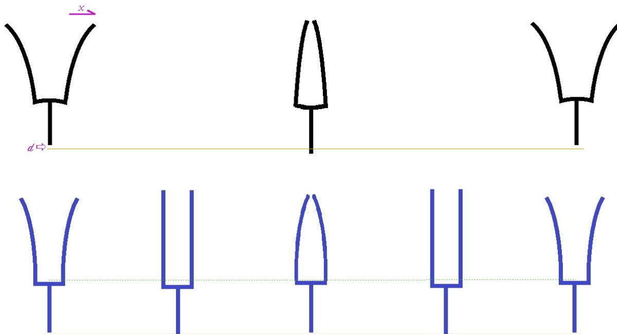
On the other hand, bending the tines lowers (very slightly) their center of mass. For all vibrational modes, we wish to fix the center of mass of the object as a whole. So if the center of mass of the *fork* remains stationary, then the stem must move up very slightly when the tines are bent... *either bent in or bent out!* If this is how the stem moves, then it will move up and down *twice* while the tines move in and out. This will create a tone an octave higher.
